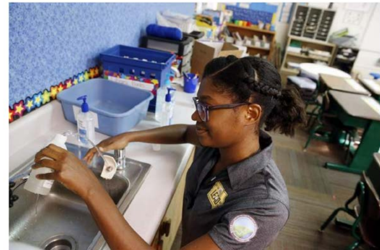
Aminia Grant, a third-year Ph.D. environmental engineering student at the University of Iowa, collects a sample from a classroom water fountain during a Nov. 23 retest for lead levels at Strawberry Hill Elementary School in Anamosa on Saturday. All faucets and fountains in the school were tested earlier this year, and the one faucet that tested above federal standards had the pipe and fixture replaced. (Liz Martin/The Gazette)
